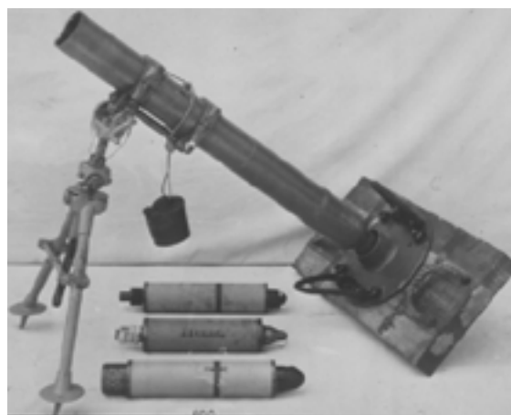
Fig. 2-11. A complete Stokes mortar with ammunition and accessories for firing. Photograph: Chemical and Biological Defense Command Historical Research and Response Team, Aberdeen Proving Ground, Md.
